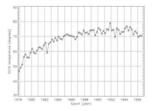
Figure 6-10. History of average engine valve 10 temperatures.
