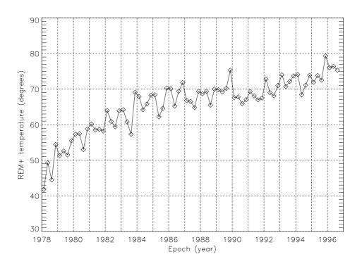
Figure 6-11. History of average remote engine module temperatures.
