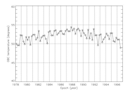
Figure 6-2. History of average onboard processor 1 temperatures.
