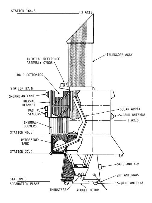
Figure 6-1. IUE Interior and Exterior Features.
