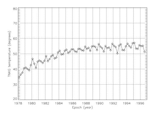
Figure 6-7. History of average hydrazine tank G temperatures.
