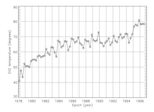
Figure 6-8. History of average engine valve 2 temperatures.
