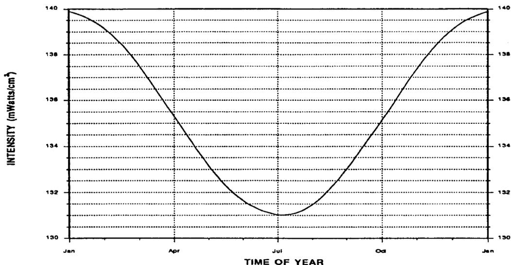
Figure 5-1. Solar Intensity vs. Time of Year.
