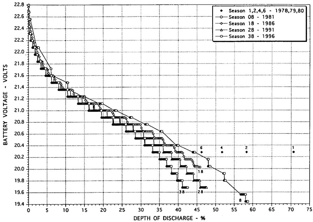
Figure 5-16. Battery 1 Voltage vs. DOD during Season 1-38.
