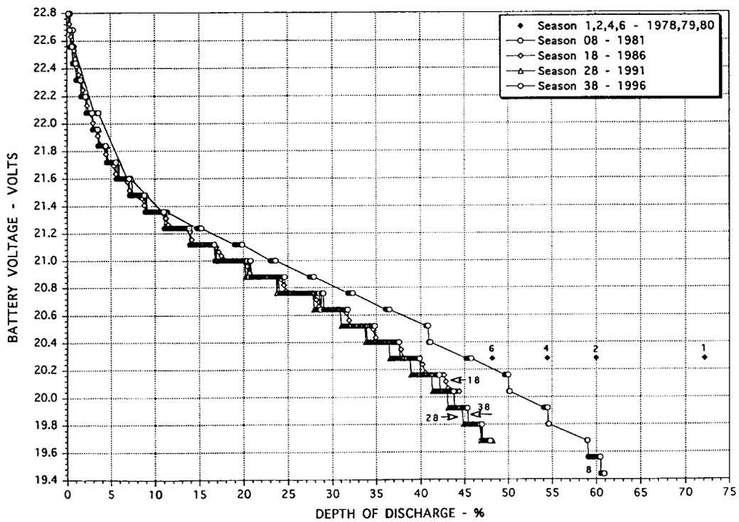
Figure 5-17. Battery 2 Voltage vs. DOD during Season 1-38.
